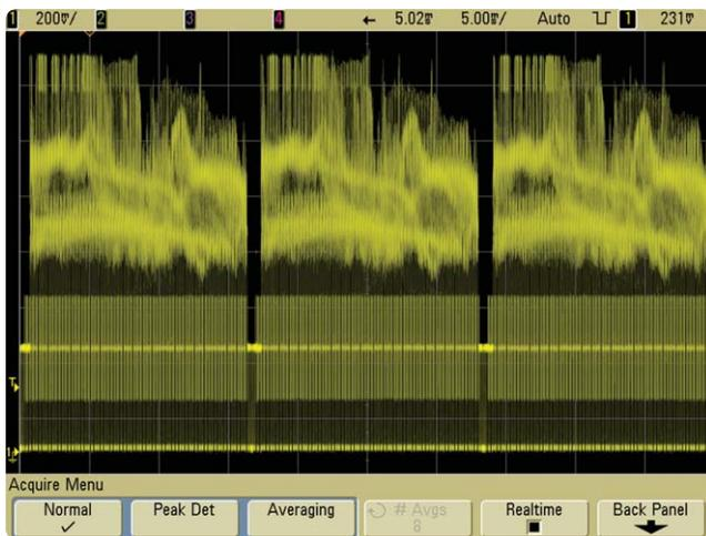
**Figure 3. Full frame of composite video displayed on Agilent's 6000 Series scope**
