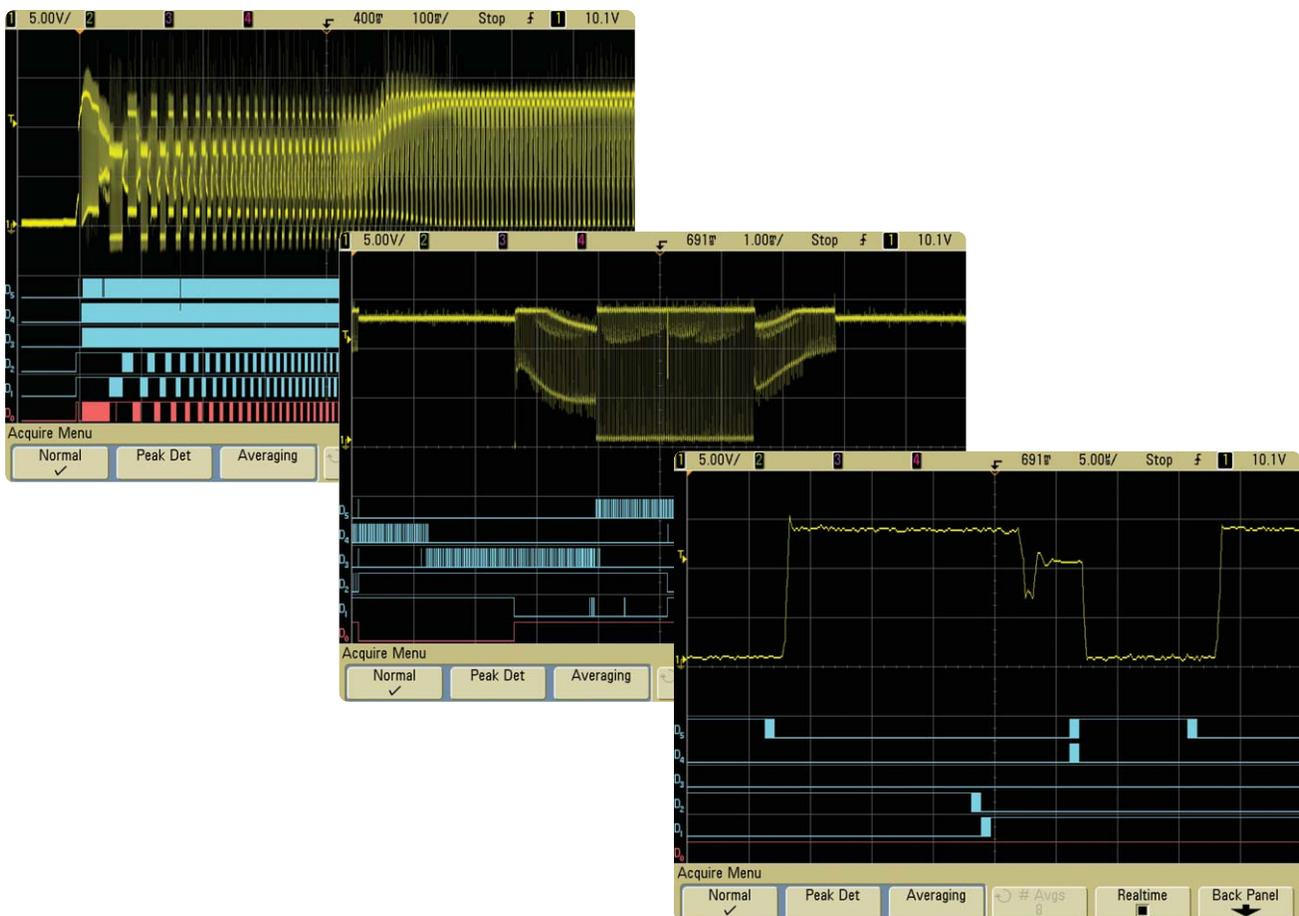
Figure 7. Motor drive signal start-up sequence with digital control signal triggering and various levels of zoom to reveal "run" pulse using Agilent's 6000 Series MSO
